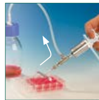
Aspiration with reverse modus valve
